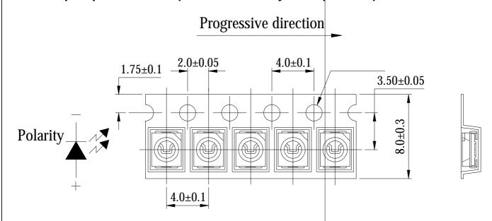
Note: Tolerance unless mentioned is ±0.1mm; Unit = mm
